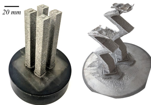
Figure 1: 10 \times 10 \times 80 \text{ mm}^3 and overhang Tungsten structures fabricated using 5kW power
