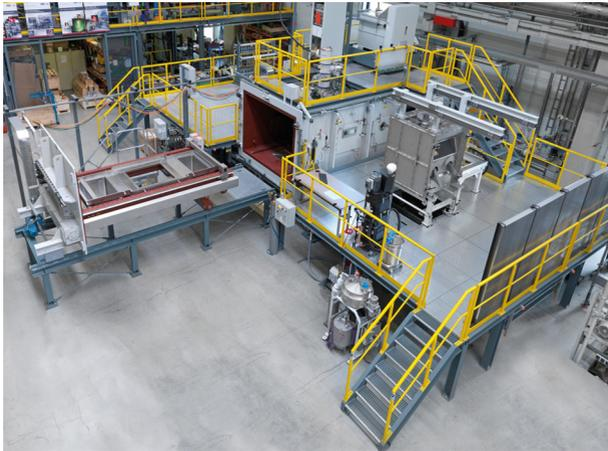
Figure 1: ALD's EBuild® 850 is the world's largest E-PBF system located in Hanau, Germany.
