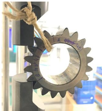
Figure 1: Tooth root bending fatigue testing of a planetary gear.
