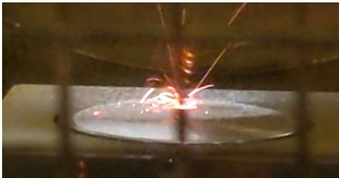
Figure 1: Electron beam melting of ball milled steel powder without preheating.
