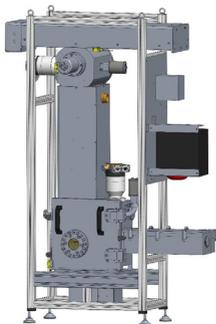
Figure 1: Schematic of the E-PBF sample environment for synchrotron studies.
