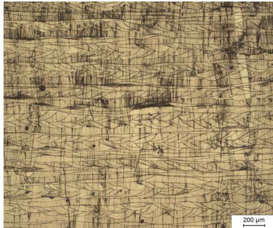
Figure 1: Microstructure of EBM-built 316L material.
