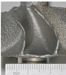
Fig. 1: A photograph of a rotor wheel showing the effect of surface finishing on one blade segment
