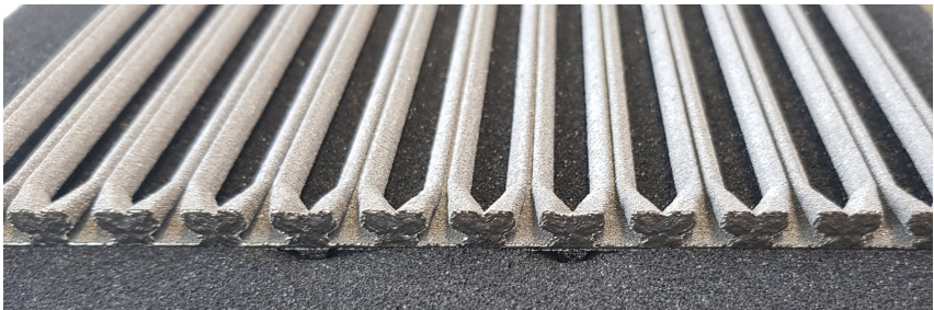
Figure 1: Pure tungsten demonstrator manufactured by electron beam melting.
